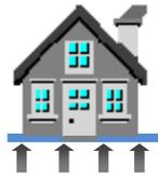
**Purpose:** Slab-on-grade installations of resilient, wood flooring, carpet, and tile when a moisture barrier is required. Proper installation will reduce moisture transmission as high as 12 lbs. to below 3 lbs per 1000sq.ft. Following information includes AQUA SEAL WATERPROOFING MEMBRANE used as the moisture barrier and UNIVERSALL PATCH as a cement top coat.
